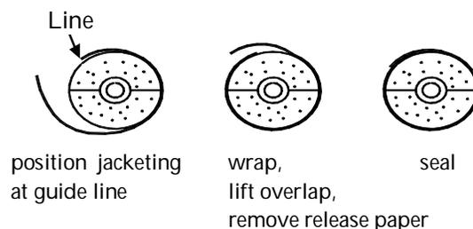
Any gaps or folds should be removed and resealed immediately. An ordinary wallpaper seam roller has been found to be particularly useful for applying pressure to the overlap areas. Note: Cure occurs in a few hours after seal is made
